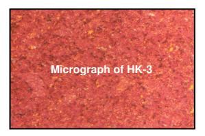
HK-3 is a premier grade of ultra-fine graphite, best used where ultra-high definition and excellent edge wear resistance are critical i.e. high quality mould making, aerospace industries and fine detailed rib forms. Good MRR rate/wear ratio. Surface finish: 16 VDI
